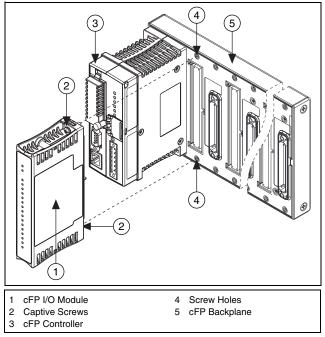
Figure 2. Installing the cFP-CTR-502
